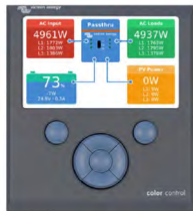
Color Control GX showing a PV application
