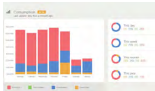
VRM Portal Our free remote monitoring website (VRM) will display all your system data in a comprehensive graphical format. System settings can be changed remotely via the portal. Alarms can be received by e-mail.
