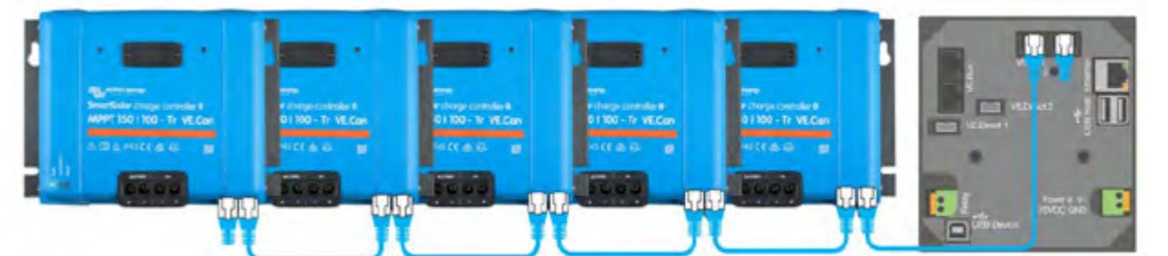
With VE.Can or Bluetooth up to 25 respectively up to 10 Charge Controllers can be daisy-chained for synchronous charging and connected to a Color Control GX or other GX device. Each Controller can be monitored individually, for example on a Color Control GX and on the VRM website (VE.Can) or on a smartphone or iPad (Bluetooth)
