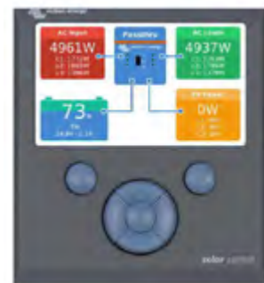
Color Control GX, showing a PV application
